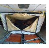
EU funding has led to the development of the first lightweight technology able to contain the devastation caused by exploding bombs hidden in airplanes' baggage compartments. The bombresistant liner-bags are strong enough to withstand the energetic effects of a blast without breaking. The linerbags have passed stringent safety tests and are ready to be installed in the cargo holds and cabins of passenger aircrafts.
